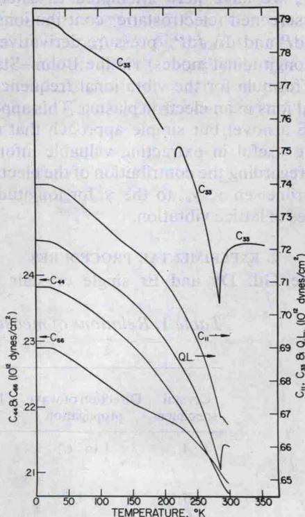
Fig. 1. Elastic moduli at zero magnetic field vs temperature for Gd, where  $T_c = 291^\circ\text{K}$ . Anomaly in  $c_{33}$  at  $\sim 215^\circ\text{K}$  is related to change in direction of easy magnetization.
